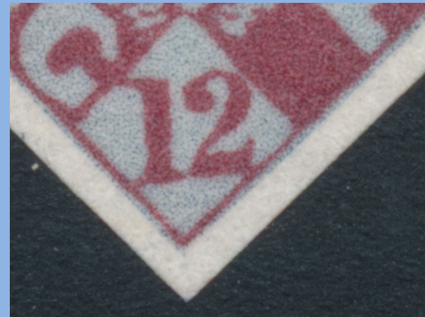
Close-up Showing 'Worm-like' Grain Pattern Typical of Collotype Process
